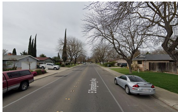
Figure 5: Edgeline Striping (Orangeburg Ave)
